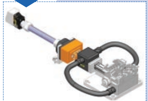
Connection system for a sequential gearbox
